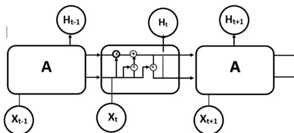
**Fig. 7 LSTM Architecture**
