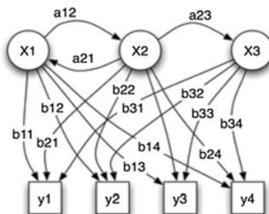
The Fig. 4 represents the hidden Markov model general architecture. In this architecture, each random variable represented as oval shape, where each random variable consists of list of values.
