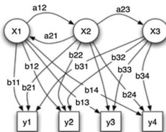
The Fig. 4 represents the hidden Markov model general architecture. In this architecture, each random variable represented as oval shape, where each random variable consists of list of values.
