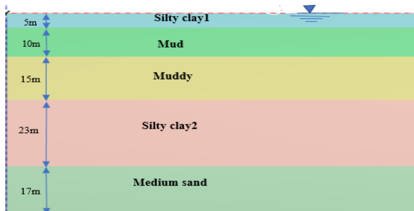
Figure (4) Soil Stratigraphy Utilized For the Case Study
