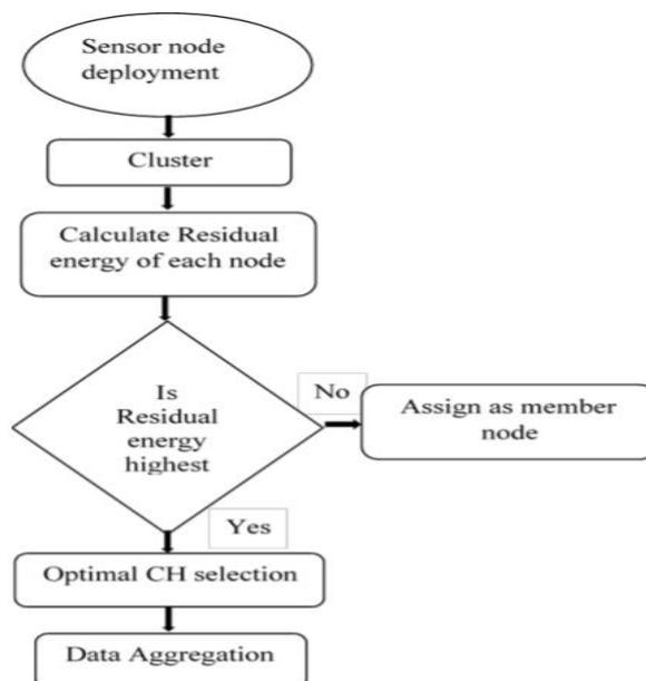
**Figure 2: Flowchart of Energy based Cluster Routing**
