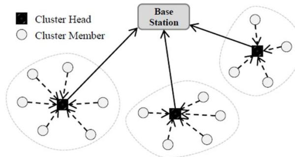
**Figure 1: Schematic Model of Cluster Based Network**
