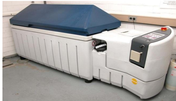
Fig 7: Salt spray test rig
