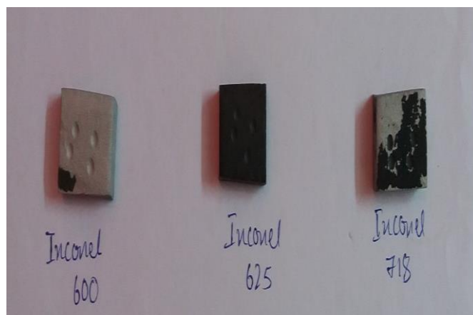
Fig 5: after Acidic Corrosion Treatment
