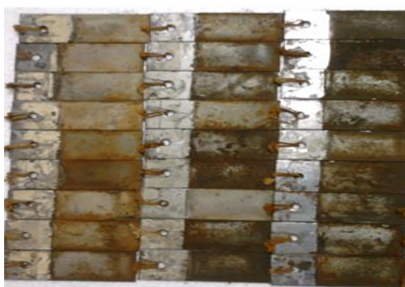
Fig 8: Cr 3 C 2 -NiCr coated Inconel Plates after Corrosion
