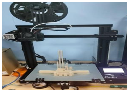
Fig 3: Fabricated test specimens built with different orientation using 3D printer
