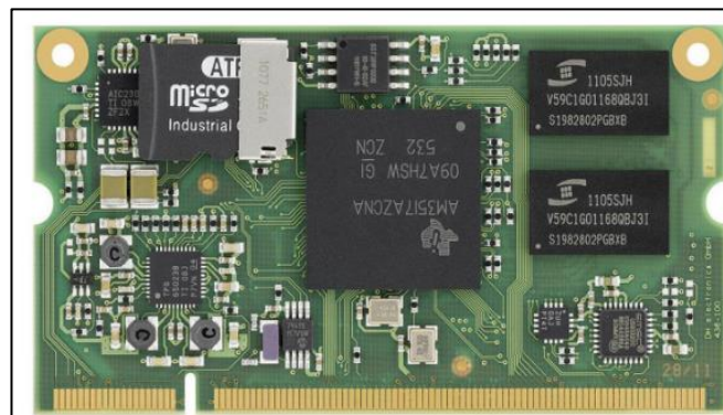
Figure 1: An integrated device with a processor, memory, and external interfaces on a plug-in card [1]
