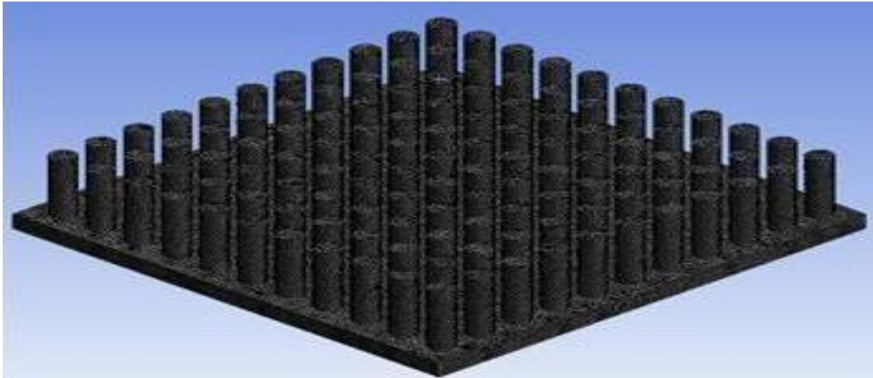
**Fig 1.02: Meshing a Heat Sink Having Hexagonal Fins**
