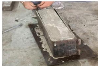
Fig 4: Demoulding of LWC block
