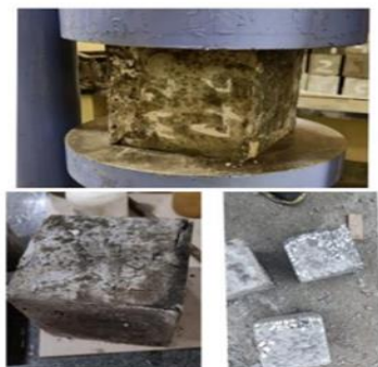
Fig 6: Testing & failure of Specimens
