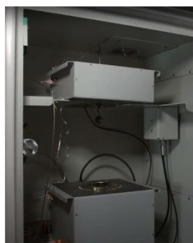
Figure 12: Set Up Of Accelerating Rate Calorimeter
