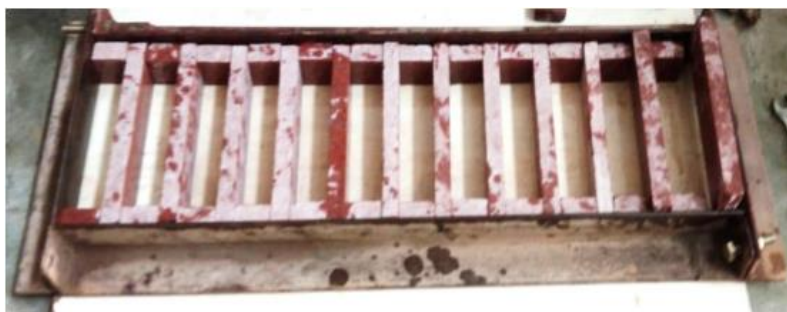
Fig 1: Mould with prism compartments
