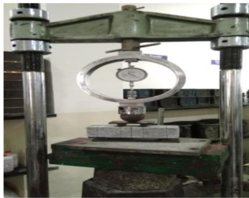
Fig 3: Flexural strength test set up
