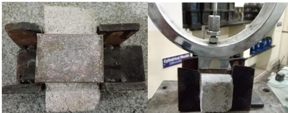
Fig 5: Compressive strength test specimen in zig and test setup
