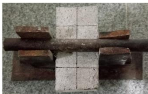
Fig 6: Tensile strength test set up
