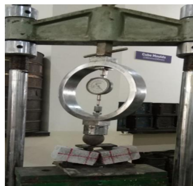
Fig 4: Flexural strength test specimen at failure
