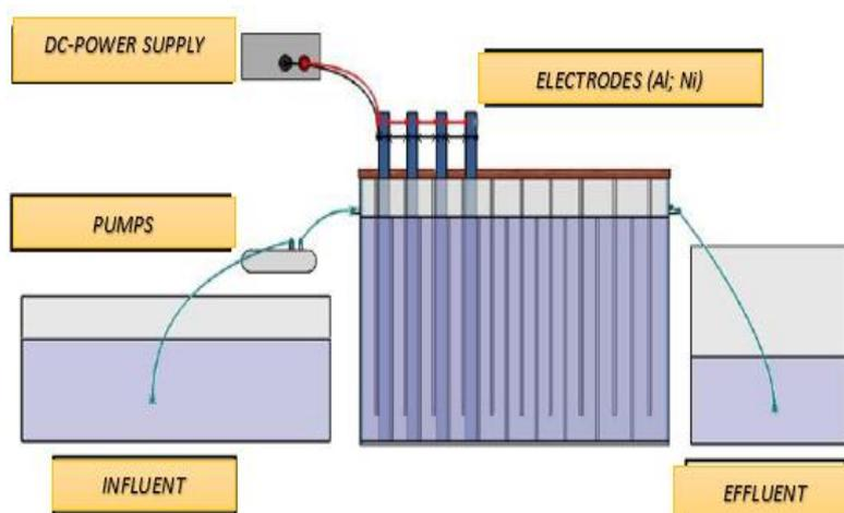
**Fig. 1: Continuous flow single channel reactor**
