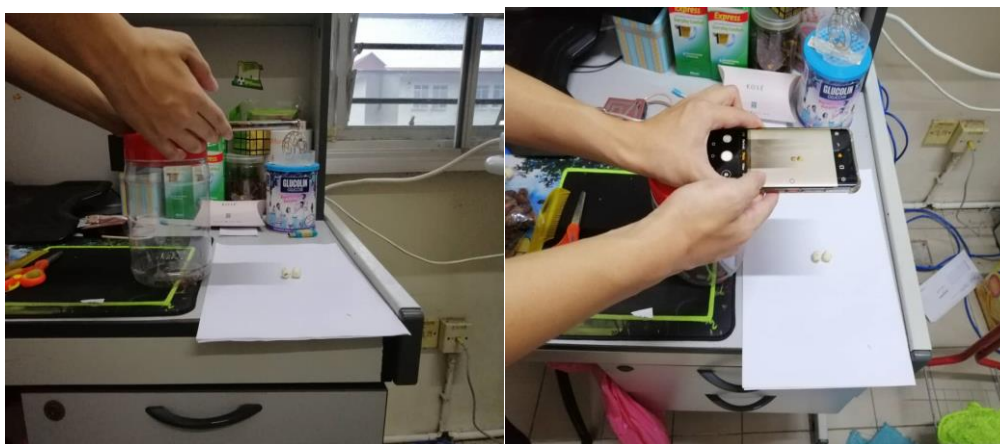
Figure 2: Fixed height of 15cm with a white background to capture the Chinese herb
