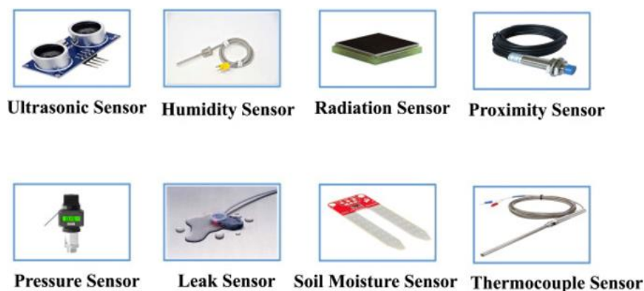
Fig 5: Smart irrigation system sensors (Source: Wikipedia)
