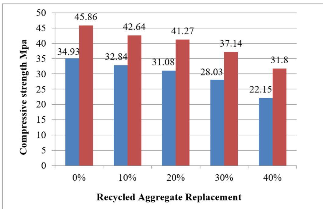
**Fig 7: 7 Days and 28 days Compressive Strength Comparison for Concrete mixes**
