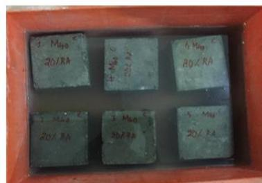
Fig 5: Cubes in chloride solution
