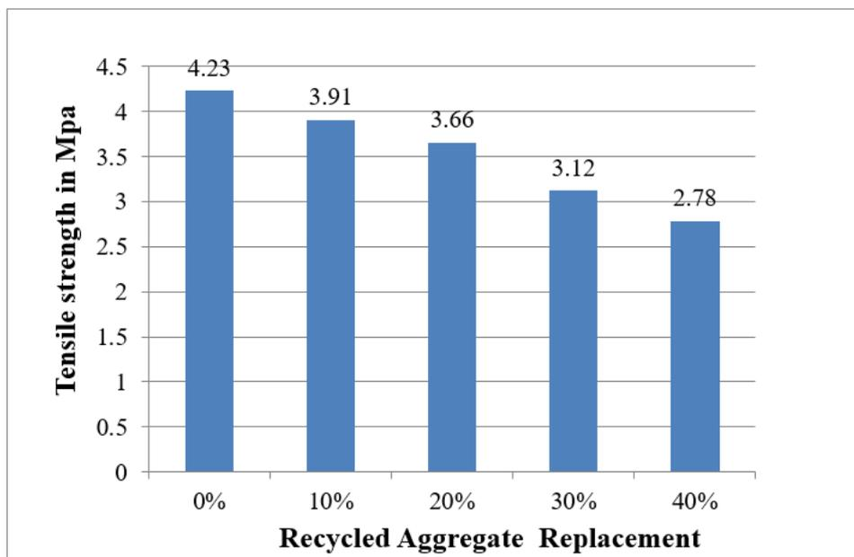
**Fig 8: Tensile strength for concrete with different % of RCA**
