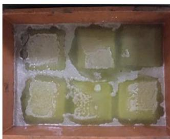
Fig 4: Cubes in acid solution
