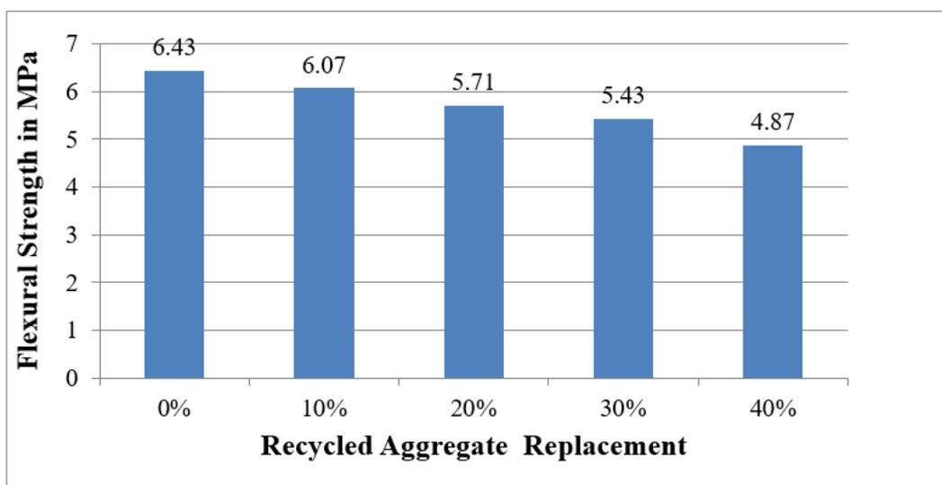
**Fig 9: Flexural strength for concrete with different % of RCA**
