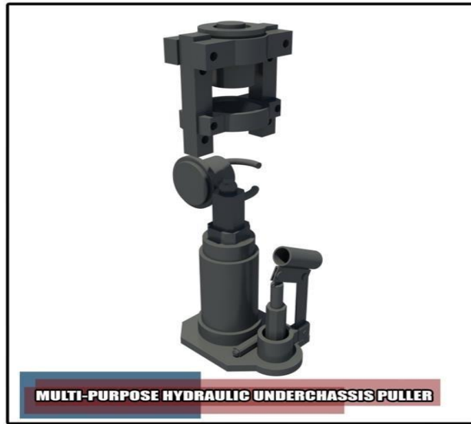
Fig 3: Multi-Purpose Hydraulic Underchassis Puller
