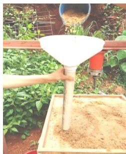
Fig 4: Sand Raining Technique using Funnel
