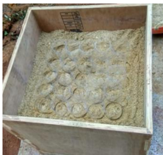
Fig 6: Reinforcement arrangement during specimen preparation
