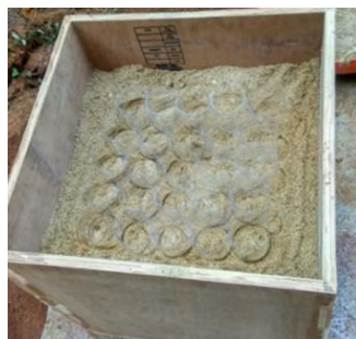
Fig 6: Reinforcement arrangement during specimen preparation
