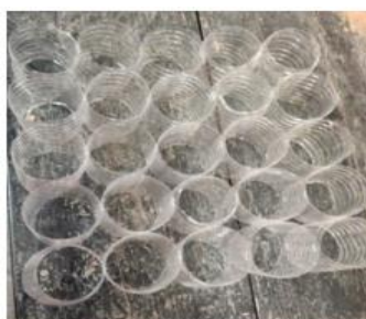
Fig 1: Reinforcement produced using plastic
