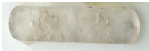
Figure 1: Bending Test Specimens for Polyester Resin Materials
