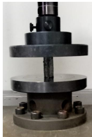
Figure 16: Compress Test of Polyester Resin Mixed with Chitosan and carbon nanodots Powder
