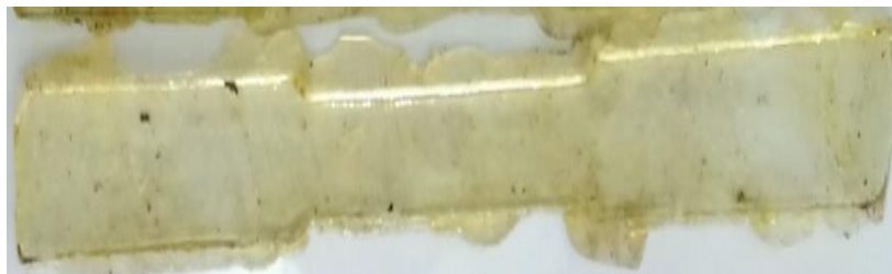
Figure 7: Tensile Test Specimens for Polyester Resin Materials
