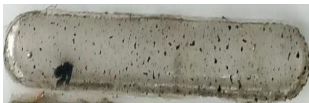
Figure 2: Bending Test Specimens of Polyester Resin Mixed with Chitosan and NanoDots (CNDs)
