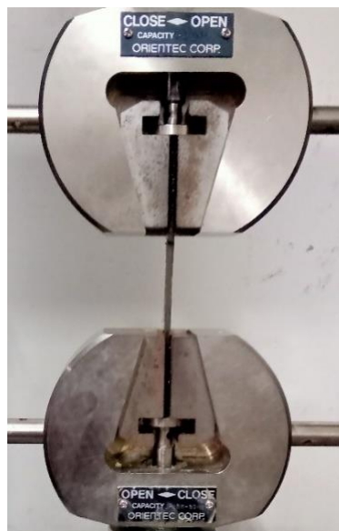
Figure 10: Tensile Test for Polyester Resin Materials Mixed with Chitosan Powder
