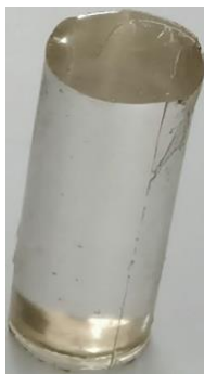
Figure 13: Specimens for Polyester Resin Materials
