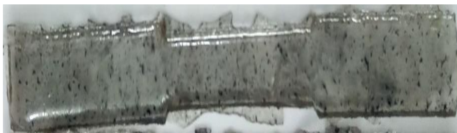
Figure 8: Tensile Test Specimens of Polyester Resin Mixed with Chitosan Powder
