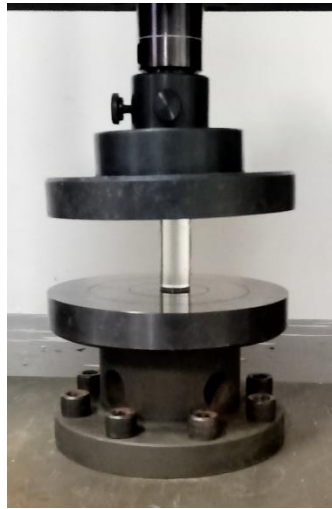
Figure 15: Compress Test for Polyester Resin Materials
