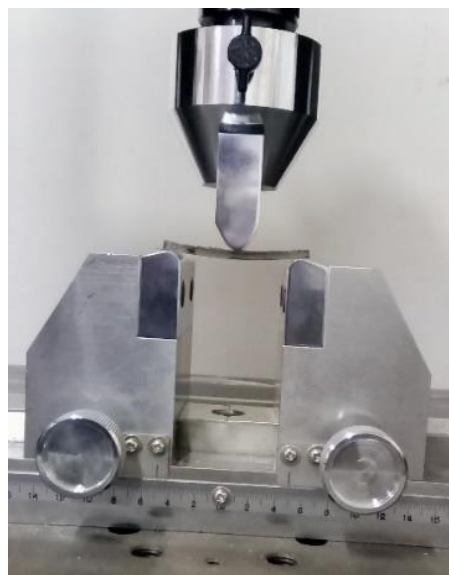
Figure 4: Bending Test of Polyester Resin Material Mixed with Chitosan and Carbon NanoDot (CNDs)
