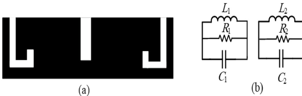
Fig 5: (a) Spurline resonator, (b) Equivalent circuit of spurlines
