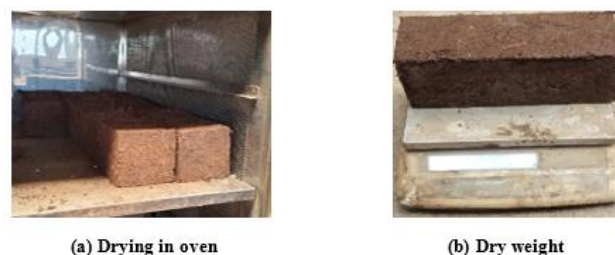
Figure 5: Determination of the dry density of SCEB
