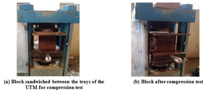
Figure 4: Compressive strength test procedure
