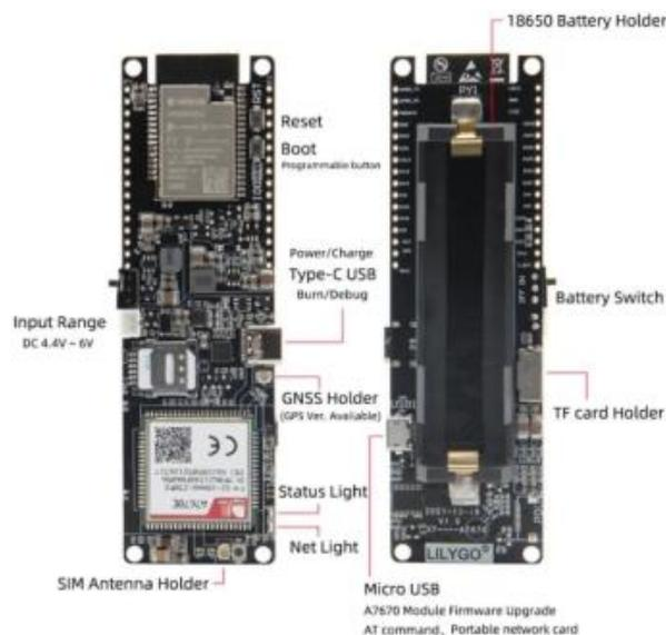
Front side: Includes the ESP32 module (central processor), Reset/Boot buttons, USB Type-C port, GNSS slot, LED indicator, antenna port, and SIM slot.
