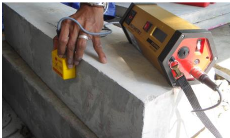
Figure 4: Mapping of reinforcement with profometer
