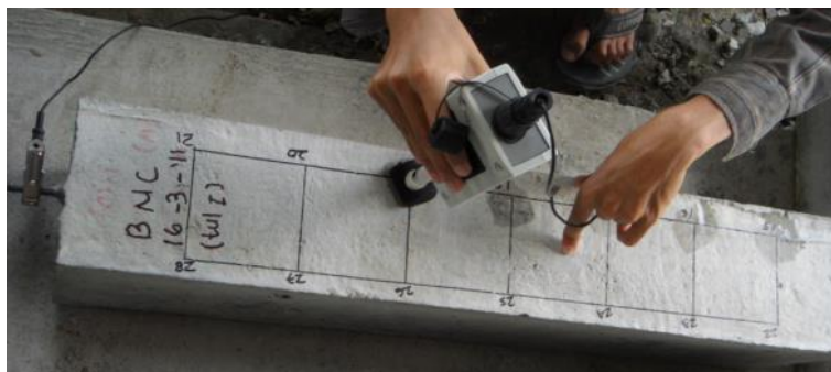
Figure 5: Set up measurement of corrosion with half-cell potential mapping
