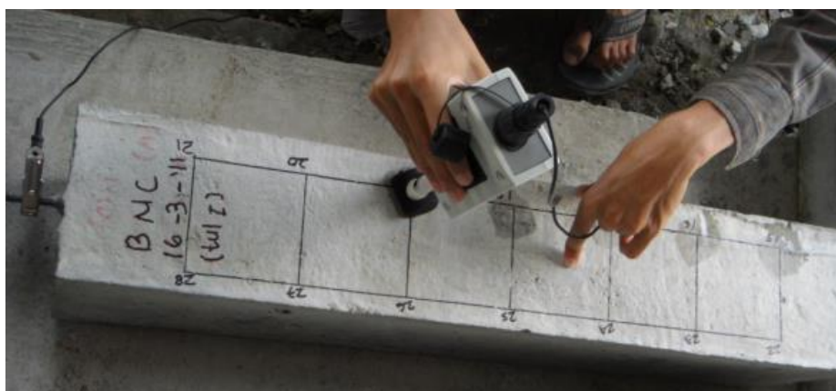
Figure 5: Set up measurement of corrosion with half-cell potential mapping
